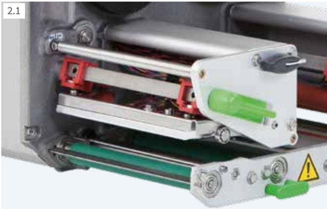
**All print heads are freely interchangeable at equal width. They are automatically detected and calibrated by the CPU. The print distance to the locating edge can be adjusted.**
